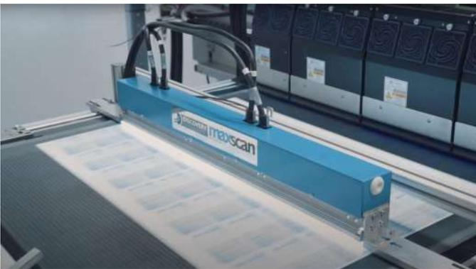
The inspection and verification of integrity marks and security features are common requirements for a wide range of web and sheet-based products, such as statements, bills & invoices as well as for bank notes, cheques, lottery tickets and software security labels. Requirements include checking the presence, position and integrity of applied features such as barcodes, QRcodes, foils and hologram devices and base paper inserts such as security threads and watermarks.
